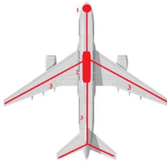
Figure 4. Fiber Optic Cable Control Block Diagram: 1 - FOSG (Fiber Optic Signal Generator). 2 - Signal Divider/Controller. 3 - Fiber-optic Bus
